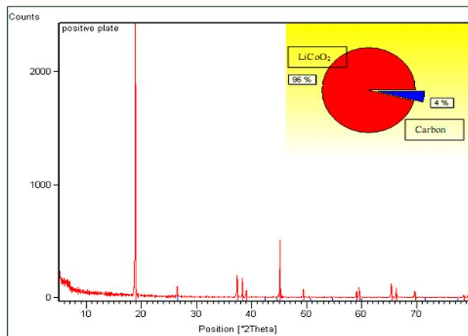
Figure 4: The XRD spectra of lithium cobalt oxide
